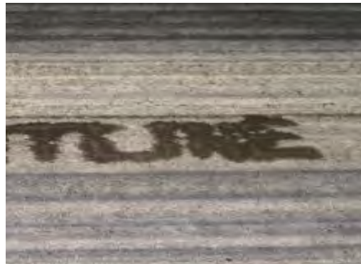
FIGURE 4-35. RUST REMOVER DAMAGED GLASS BEADS, MAKING THEM INEFFECTIVE.
