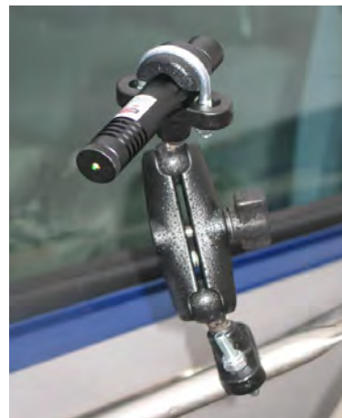
FIGURE 6-56. PORTABLE LASER POINTER.
