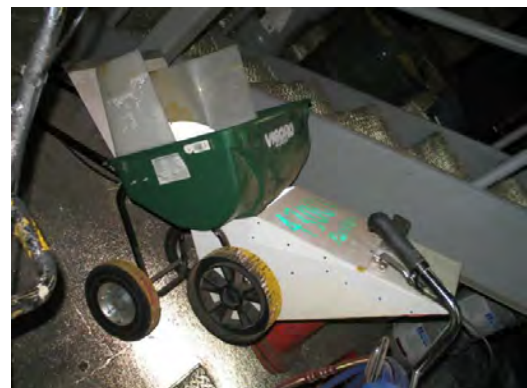
FIGURE 6-36. FERTILIZER SPREADER WAS MODIFIED TO APPLY GLASS BEADS.
