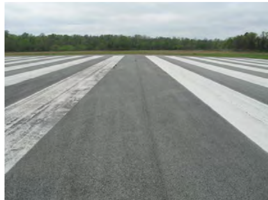
FIGURE 4-23. SAME MARKINGS AS IN FIGURES 4-21 AND 4-22, AFTER THIRTY MONTHS.
