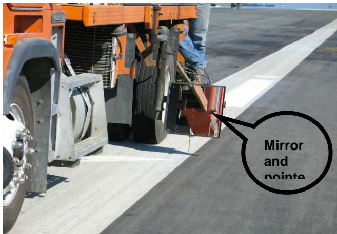
FIGURE 6-55. POINTER WITH MIRROR.
