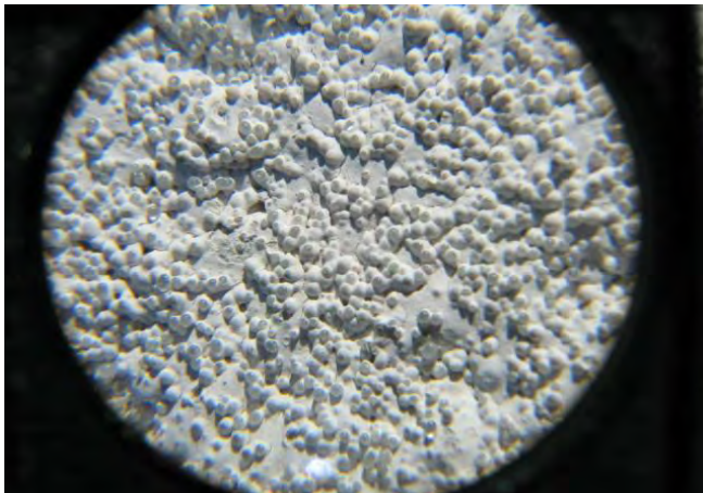
FIGURE 6-64. EXCESSIVE WICKING OF PAINT OVER BEADS.
