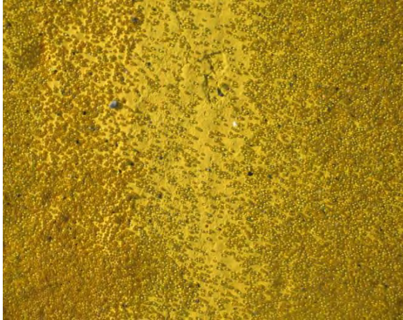
FIGURE 3-9. TYPE IV BEAD DISTRIBUTION IS POOR.
