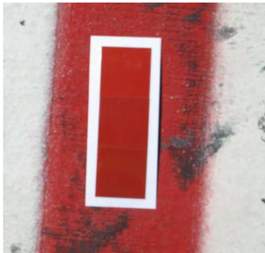
FIGURE 6-70. RED COLOR CHIP COMPARED TO RED MARKING.
