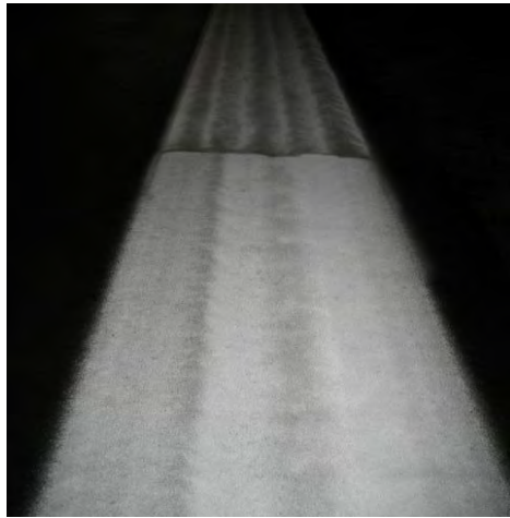
FIGURE 6-31. PRESSURIZED BEAD APPLICATION IN FOREGROUND, GRAVITY-DROP IN BACKGROUND.
