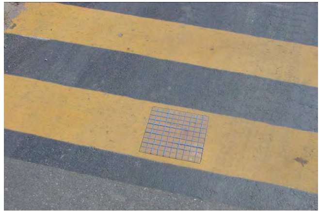
FIGURE 6-72. GRID FOR COMPLIANCE WITH DEGREE OF PAINT REMOVAL.
