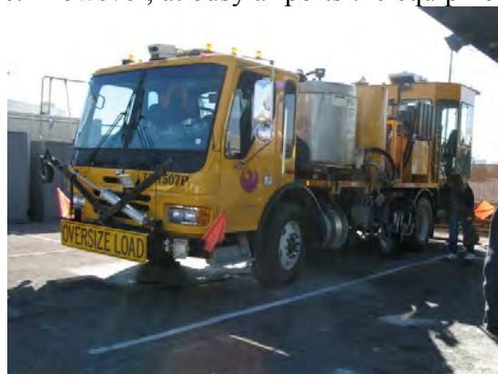
FIGURE 6-24. TRUCK-MOUNTED AIRPORT STRIPING EQUIPMENT.
