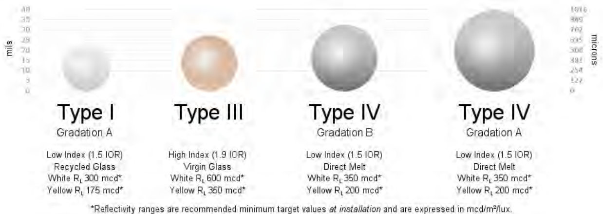
FIGURE 3-4. SIZE COMPARISON OF GLASS BEADS FOR AIRPORTS
