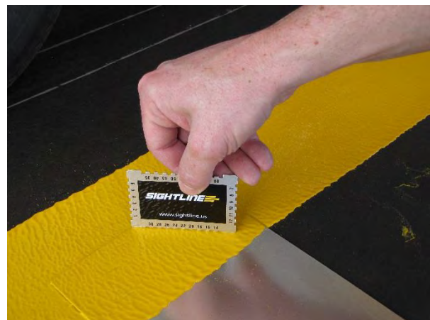
FIGURE 6-62. USE OF WET FILM GAUGE.
