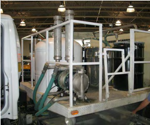
FIGURE 6-29. PNEUMATIC TRUCK-MOUNTED SYSTEM.
