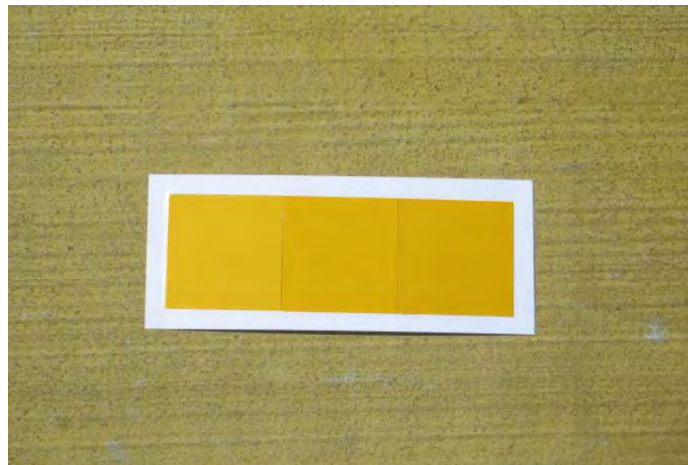
FIGURE 6-71. YELLOW COLOR CHIP COMPARED TO YELLOW MARKING.
