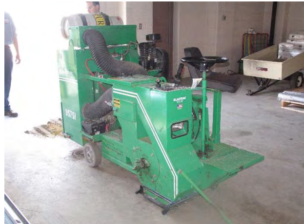
FIGURE 5-13. SHOTBLASTER WITH A 10-INCH CUT.
