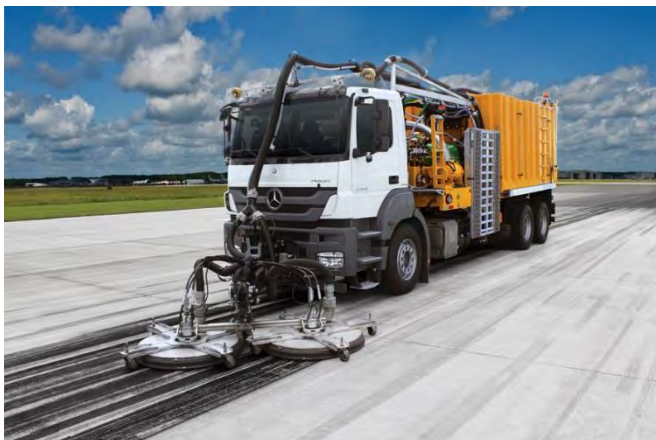
FIGURE 4-47 – ULTRA-HIGH-PRESSURE WATERBLASTER WITH 6-FOOT PASS AND FULL WATER RECOVERY.
