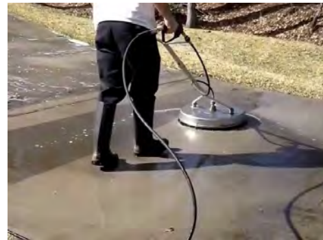
FIGURE 4-43 - PRESSURE WASHER WITH FLOOR ATTACHMENT
