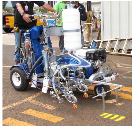
FIGURE 6-39. AN AIRLESS MACHINE WITH PRESSURIZED GLASS BEADS.
