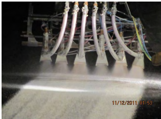
FIGURE 6-18. PNEUMATIC PAINT GUNS AND GLASS BEAD GUNS MOUNTED TO TRUCK ON CARRIAGE.
